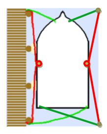
The powerboat lies against two pilings, and has a midship cleat. Spring lines are run fore and aft from that cleat to pilings off the bow and stern.
