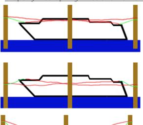
A view from the side shows how a boat with properly tied spring lines and bow and stern lines will look at low tide and high tide. Note that the lines are attached to the piling at the level of the boat during a medium tide, so that they rise up to the boat for high tides and fall down to it for low tides.
